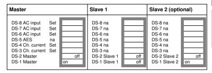
The current settings (AC current limitation and charging current) are multiplied by the number of devices. However, the AC current limitation setting when using a remote panel will always correspond to the value indicated on the panel and is **not** multiplied by the number of devices.
