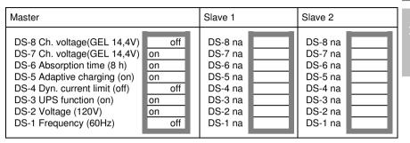
To store the settings after the required values have been set: press the 'Down' button of the **master** for 2 seconds (**lower** button to the right of the DIP switches). **The temperature and low-battery LED's will flash to indicate acceptance of the settings**.
