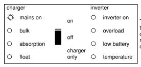
The AC input is switched through. The AC output current is equal to the preset maximum input current. The charge current is reduced to 0.
