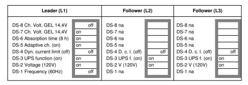
To store the settings after the required values have been set: press the 'Down' button of the **leader** for 2 seconds (**lower** button to the right of the DIP switches). **The temperature and low-battery LED's will flash to indicate acceptance of the settings**.
