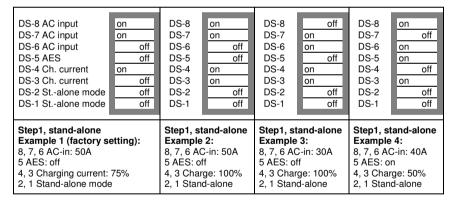
To store the settings after the required values have been set: press the 'Up' button for 2 seconds (upper button to the right of the DIP switches, see appendix A, position J). The overload and low-battery LED's will flash to indicate acceptance of the settings.
