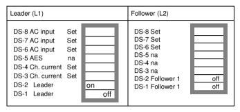
As the table above shows, the current limits for each phase should be set separately (ds8 thru ds5). Different current limits per phase can be selected.
