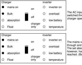
The AC input voltage is switched through and the charger operates in bulk mode.
